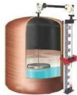
Float & Board Type Level Indicator
